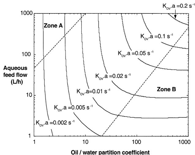
**Figure 12. Configuration 1: overall volumetric mass-transfer coefficient as a function of operating conditions (Zone A: more than 80% of the overall resistance to mass transfer is located in the membrane; Zone B : more than 80% of the overall resistance to mass transfer is located in the shell-side).**
