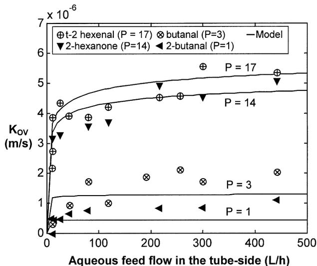
**Figure 7. Overall mass-transfer coefficient vs. aqueous feed flow in the tube side.**
