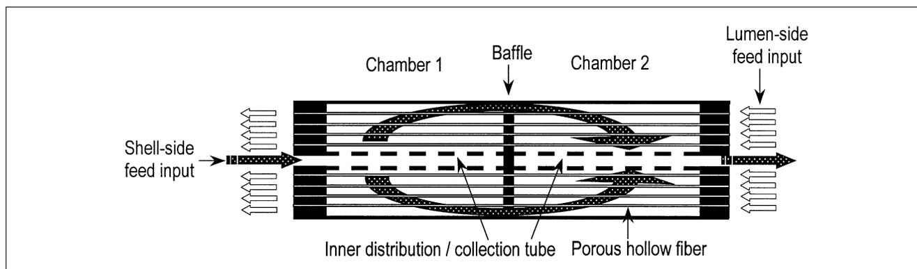
Figure 2. Licicel Extra-Flow hollow-fiber contactor.
