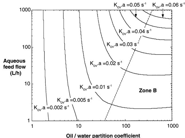
**Figure 13. Configuration 2: overall volumetric mass-transfer coefficient as a function of operating conditions (Zone B: more than 80% of the overall resistance to mass transfer is located in the tube side).**
