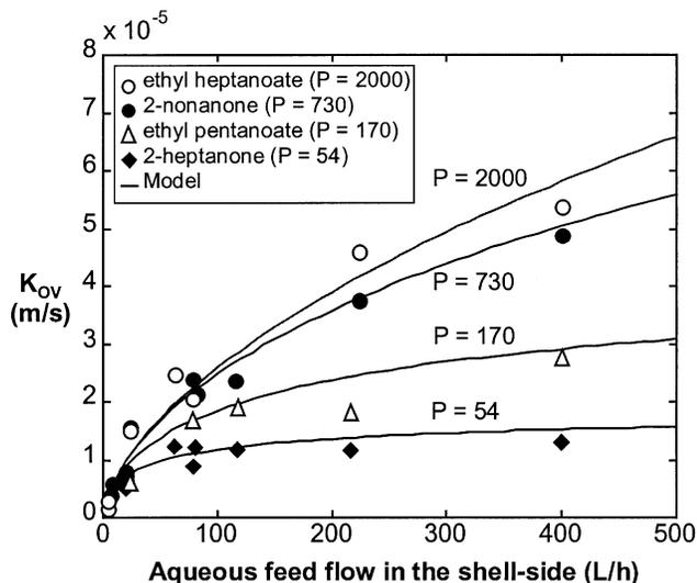
**Figure 4. Overall mass-transfer coefficient vs. aqueous feed flow in the shell side.**
